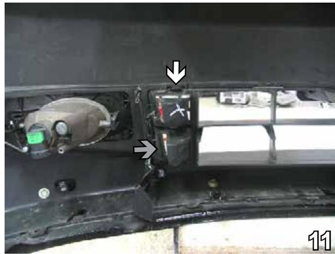
11. On the driver's side, mark the upper air vent flush with the back side of the grille opening. Using the utility knife, trim the marked area. Some models may need to have the lower air vent removed also (see grey arrow).
