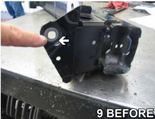
9. Flatten bumper bracket with a hammer.
