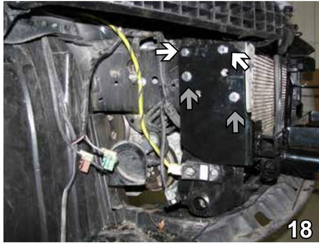
18. On the passenger side upper two holes, install 3/8-16 x 1" hex bolts from the upper frame webbing. Apply loctite and tighten to the 3/8" lock washers and 3/8-16 hex nuts on the outside of baseplate (see white arrows). Insert 3/8-16 nut plate through frame end hole and align to the bottom holes (see grey arrows). Install 3/8-16 x 1 1/2" hex bolt with 3/8" lock washer, apply loctite and tighten to the nut plate.
