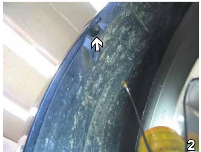
2. Just inside wheel well, on edge of fascia, remove one Phillips screw. Do this to both sides of the vehicle. Set screws aside to be reinstalled later.
