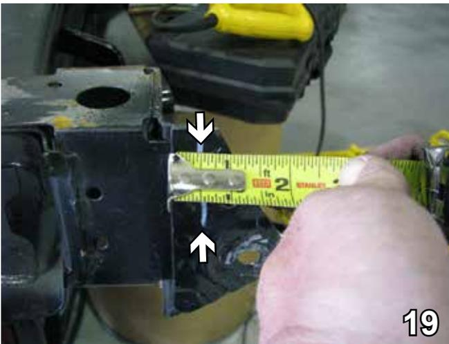
19. On the passenger side only, trim the side of the metal bumper, Measure 3/8" from the edge on the top and cut straight down. Reinstall the bumper.
